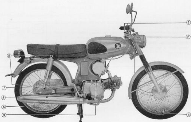
Fig. 5.40 Torquing points on right side
