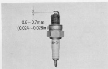
Fig. 5.10 Measuring spark gap
