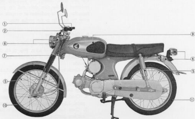
Fig. 5.45 Daily inspection points on left side
