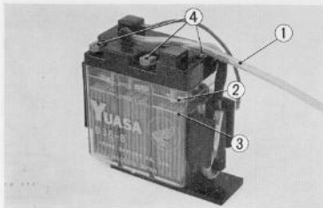
Fig. 5.37 Battery electrolyte level ① Vent pipe ② Upper level mark ③ Lower level mark ④ Filler cap
