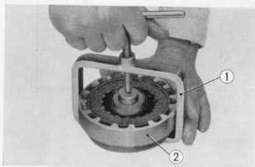
Fig. 3.67 Disassembling the clutch ① Clutch disassembling and assembling tool ② Clutch assembly
