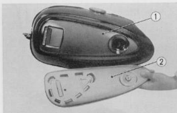
Fig. 4.43 Removing tank side cover ① Fuel tank ② Tank side cover
